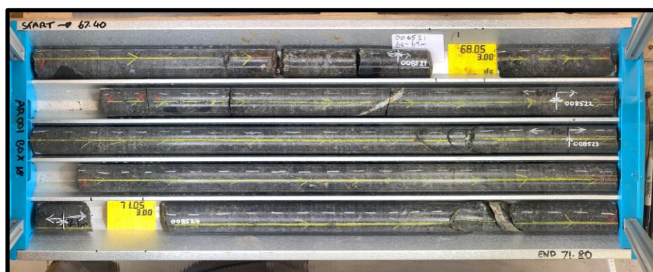
Picture 3: Example of the rock cores recovered from mineral drilling.
