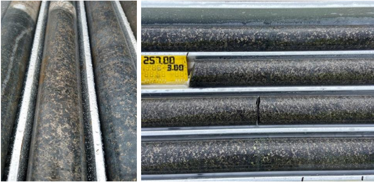
Examples of net-textured sulphides intersected in 2024 drilling. Left – AR011DD at 227 metres. Right – AR016DD at 257 metres.
